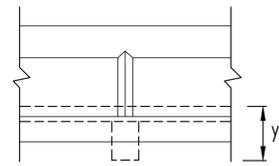
DETALLE II CORTE B-B (DIENTES EN LOS ESTRIBOS Y LOSA)
